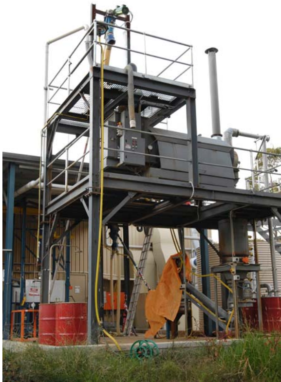
Rotary kiln (Sulphation)
